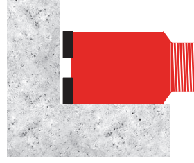
Drilling flush to the floor
